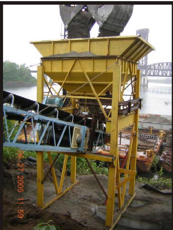
Photo 17 Sand being loaded into the hopper from the barge.
