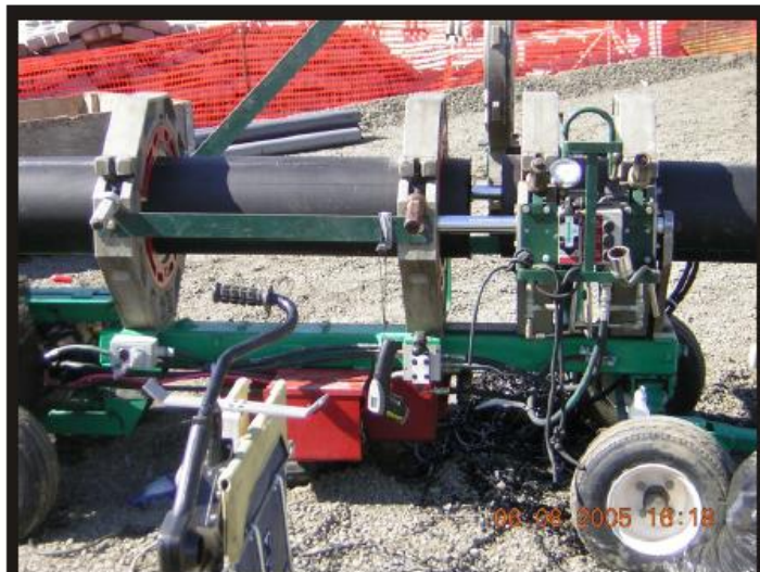
Photo 10 Welding apparatus used for joining HDPE smooth wall interior conveyance pipe sections.
